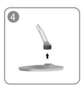
Take the Stand Connector out of the Stand by pulling it in the direction of the arrow as shown in the figure.
